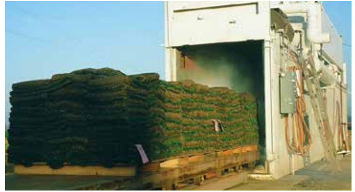
SOD is placed onto a rail car, which is pushed into the vacuum chamber. As the vacuum is drawn down the sod cools evenly throughout the pallet.
